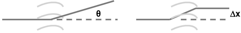
FIGURE 2: (Left) The deflection of an optical beam by an acoustic field. (Right) Two deflections in the acoustic field create an optical displacement of the beam.
